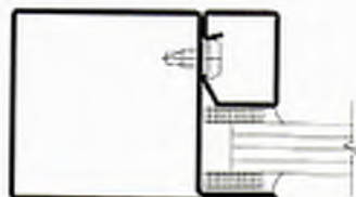
Standard profile with silicone beading (internal or external application)
